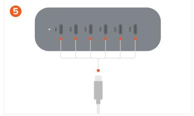
Plug in cables (sold separately) to the charger's USB-C PD ports. We always recommend using certified charging cables. EMARK cables are required to reach wattage above 60W.
