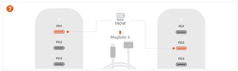
When connected to PD1 or PD2, supported device can charge with a max output of 140W. Only one device can be connected at a time to either port in order to achieve 140W charging. USB-C to MagSafe 3 Cable must be used in order to achieve 140W output through PD1 or PD2.
