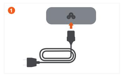
Connect the included C5 power cable to the C5 connector on the rear of the charger.
