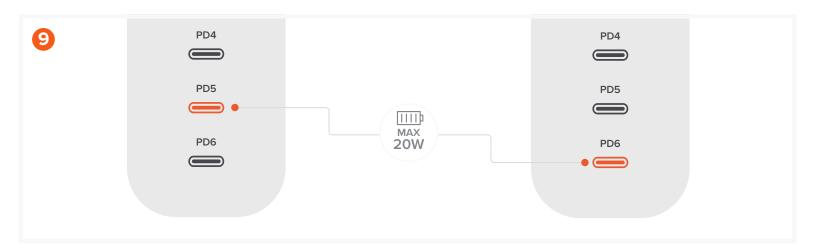
When connected to PD5 or PD6, supported device can charge with a max output of 20W.
