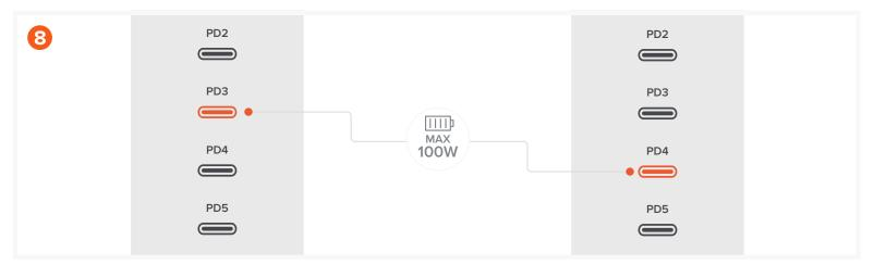
When connected to PD3 or PD4, supported device can charge with a max output of 100W.
