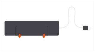
Insert the SSD (not included) faceup with the pins aligned and push down on the screw to secure it into place. Supports SATA M.2 SSD only, does not work with Nvme
