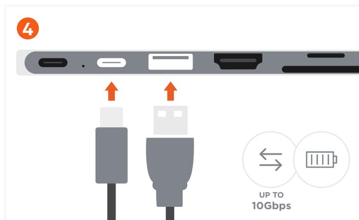
4 Use the USB-C and USB-A ports for fast data transfer speeds - up to 10Gbps
