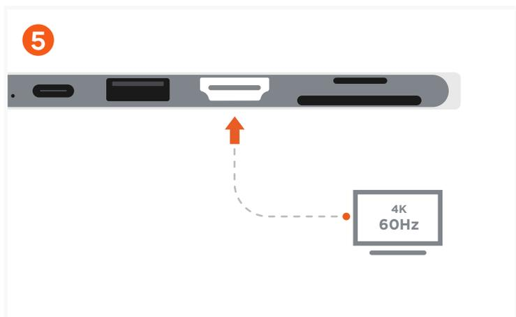
5 Use the HDMI port to output up to 4K / 60Hz with an external monitor.
