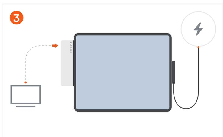
3 When using the USB4 port for video output, it is recommended to use the proprietary charger to keep the Surface Pro 9 charged unless your connected monitor supports charging.
