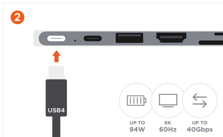
2 Use the USB4 port to charge your device up to 94W, output video up to 6K/60Hz, or transfer data up to 40Gbps.
