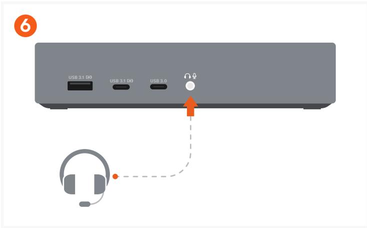
Attach audio device to 3.5mm Audio I/O jack. You will need to change sound output/input settings when connecting headphones/mic. (System Preferences > Sound > Output/Input > USB Audio).
