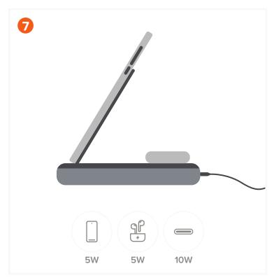
When both wireless chargers and USB-C port are being used to charge devices, the power bank will support the following output power schematic:
