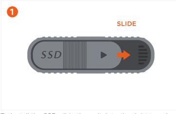
To install the SSD, slide the switch to the right to unlock the top door of the enclosure.
