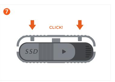
Press the opposite side to latch. You should hear a clicking sound signifying that the enclosure top is locked into place.
