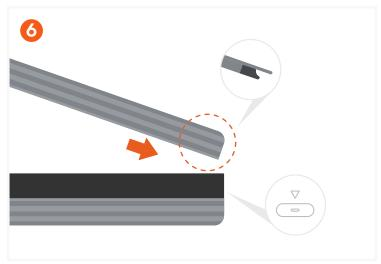
To reinstall the top cover align the side with the metal hooks toward the USB-C port.
