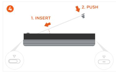
Insert the SSD (*not included*) at an angle and faceup with the pins aligned and push down on the silicone pin to secure it into place.
