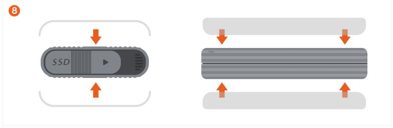
To reinstall the included case press it into place.
