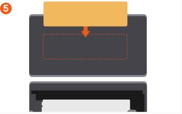
To apply the included thermal pad peel the blue film and attach the pad to the top cover of the enclosure. Remove the clear film from the thermal pad before closing the enclosure
