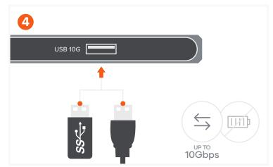
USB 3.2 Gen 2 port allows for transfer data at up to 10Gbps speed. Does not support charging or Apple SuperDrive.
