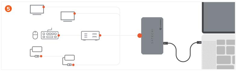
Allows for daisy-chaining up to 6 devices
