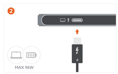
Using the included Thunderbolt 4 cable, connect the hub to your host device from its Thunderbolt 4 host port located at the front of the hub. Once the host device is connected, the LED color will change to green. Features 96W max pass-through charging to the host device.
