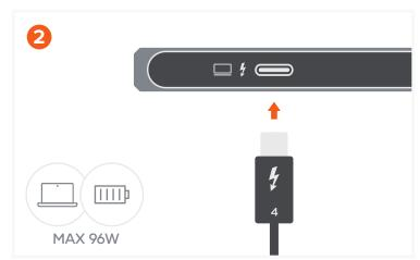
Using the included Thunderbolt 4 cable, connect the hub to your host device from its Thunderbolt 4 host port located at the front of the hub. Once the host device is connected, the LED color will change to green. Features 96W max pass-through charging to the host device.
