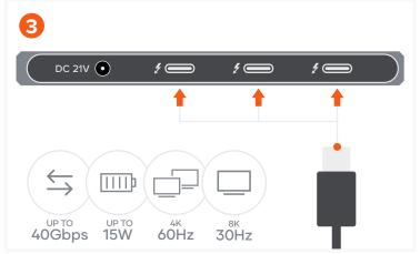
Connect up to three USB-C devices to the hub's Thunderbolt 4 ports. Supports up to 40Gbps, 15W charging, dual 4K video output up to 60Hz total or single 8K video output at 30Hz. macOS doesn't support 8K video output.
