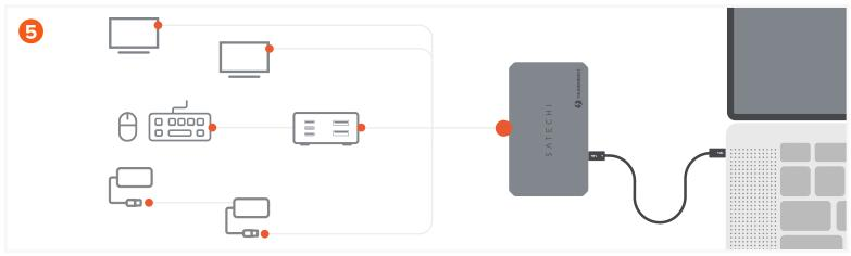
Allows for daisy-chaining up to 6 devices
