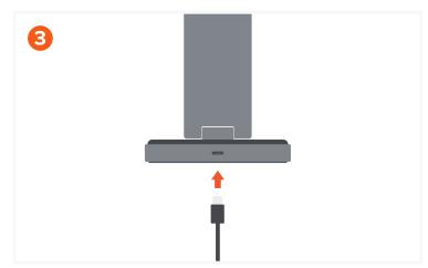
Connect the USB-C cable to the rear USB-C port on the Charging Stand. The front LED indicator will illuminate once connected to power.
