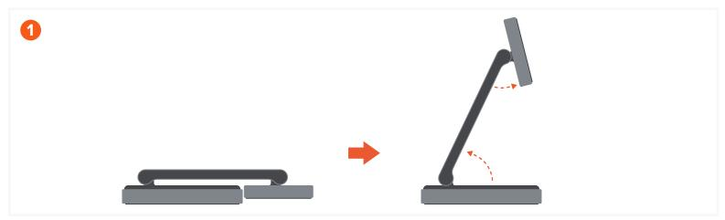
Unfold the 2-in-1 Charging Stand to an upright position.
