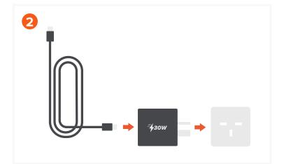
Connect the USB-C charging cable (included) to a power adapter (not included).  $\label{eq:connection}$
