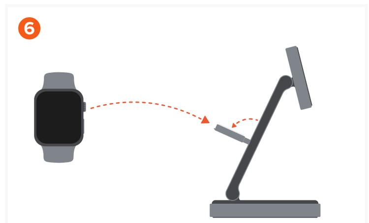
Fold down the Apple Watch module and place the Apple Watch onto it to begin charging. Supports 5W fast charging on Apple Watch Series 7, 8, 9, Ultra, and Ultra 2.
