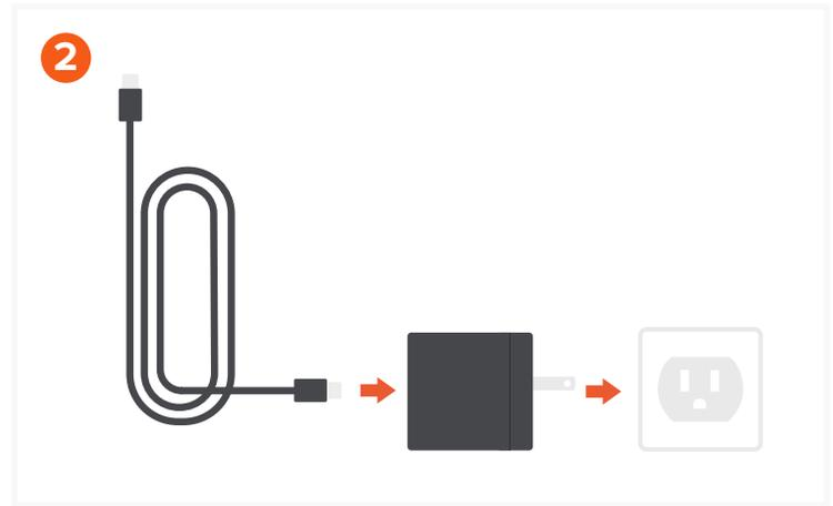
Connect the USB-C charging cable (included) to the 45W power adapter (included). Attach included wall plug adapter depending on your region. At least 36W Power Adapter required for optimal use.
