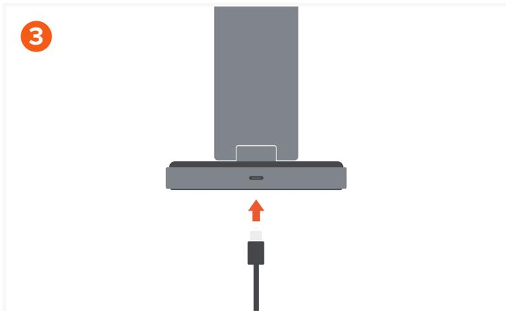
Connect the USB-C cable to the rear USB-C port on the Charging Stand. The front LED indicator will illuminate once connected to power.
