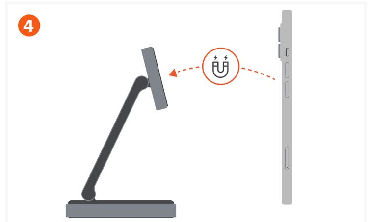
Place compatible iPhone on the Qi2 charger to begin charging. Supports charging speeds of up to 15W.
