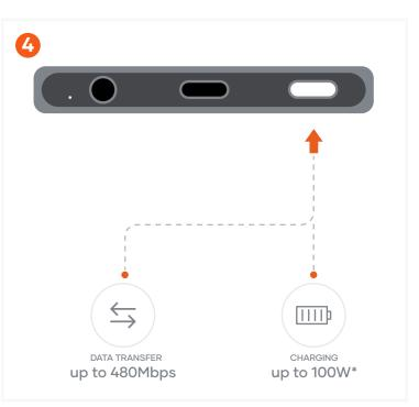
Connect a USB-C charging cable to either USB-C PD port.
