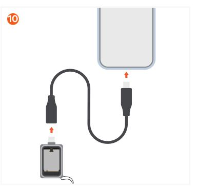
Connect the female end of the extension cable to the USB-C connector of the enclosure and the the USB-C end of the cable to your host device (e.g., computer, hub, dock, or adapter).
