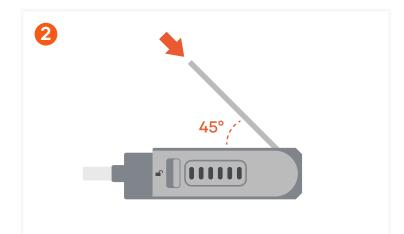
Install a 2230-sized SSD (not included) at a 45° angle. Only compatible with 2230-sized NVMe drives.
