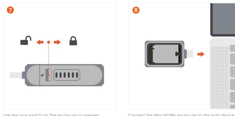
Use the lock switch on the enclosure to prevent rewriting or deletion of files.
