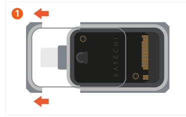
Slide to remove the magnetic cover from the enclosure.
