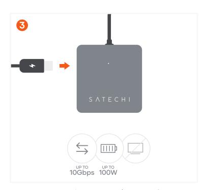
Connect power to the USB-C PD/Data port for charging.
