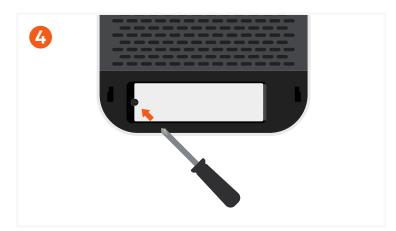
Secure the SSD using the included screwdriver and screw. Tip: To prevent stripping the screw, do not overtighten.
