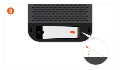
Insert the SSD at a slight angle (35-45°) and ensure it is fully seated in the PCle slot.
