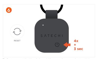
To factory reset the Keychain, quickly press the power button 4 times, then long-press for at least 3 seconds, then you will hear a beep confirming the Keychain has been reset.
