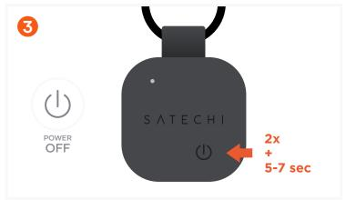
To power off the Keychain, quickly press the power button 2 times, then long press the 3<sup>rd</sup> time for at least 5 to 7 seconds. You will hear two beeps, indicating your FindAll™ Keychain is powered off. When device is powered off, you cannot track its location.
