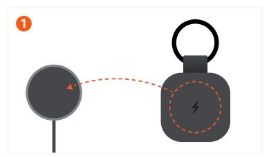
Charge the Keychain with a wireless charger (not included). The status light will be orange while charging and green when fully charged. It is recommended to charge once every 8 months. Battery life lasts up to 12 months\* on a single charge (may vary depending on usage).
