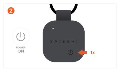
To power on the Keychain, press the power button once. It will beep to indicate it is on.
