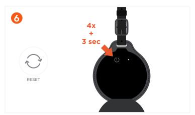
To factory reset the Luggage Tag, quickly press the power button 4 times, then long-press for at least 3 seconds, then you will hear a beep confirming the Luggage Tag has been reset.
