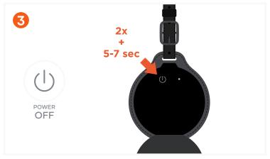
To power off the Luggage Tag, quickly press the power button 2 times, then long press the 3<sup>rd</sup> time for at least 5 to 7 seconds. You will hear two beeps, indicating your FindAll™ Luggage Tag is powered off. When device is powered off, you cannot track its location.
