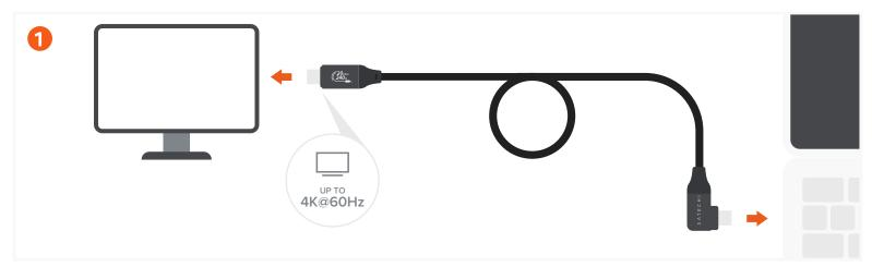
Connect the Right-Angle USB-C Data & Charge Cable to a USB-C or Thunderbolt external monitor.
