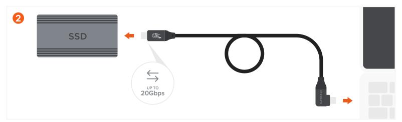
Connect the Cable to the USB-C port on your compatible host device for fast data transfer speeds up to 20Gbps maximum.
