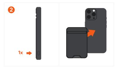
Turn on the power bank by pressing the side button once or attaching your phone. The LED lights will turn on for 14 seconds and then turn off. The power bank supports wireless charging for one device at a time.
