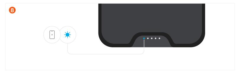
When a device is charging, the Blue LED light will remain solid, confirming the device has been detected and is charging properly.
