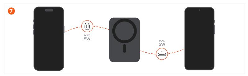
When charging two devices simultaneously (wireless + USB-C), the output will follow this configuration: Qi2 Charger (5W) + USB-C Output (5W)
