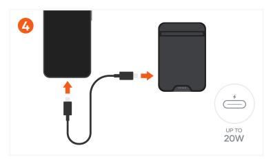
Use the USB-C port to recharge the power bank or charge USB-C tablets or smartphones.
