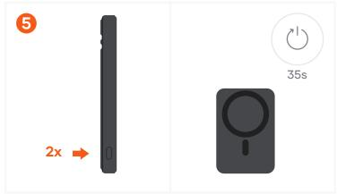
To manually power off the power bank, double-press the power button. The LED battery indicators will turn off. The power bank also features an auto-shutoff function, which activates after 35 seconds of inactivity or if no connected device is detected.
