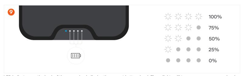
LED indicators on the back of the power bank display the current battery level. These lights will turn on upon power on showing the battery level and will remain on while charging.
