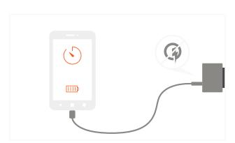
4 Connect an USB-A cable to the adapter's Type-A port to charge another USB device. Max output: 12W
