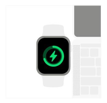
4 Remove Apple Watch from module when fully charged.
