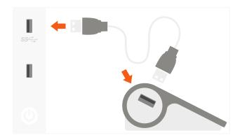
2 Connect up to 4 USB devices like external hard drives, cameras, flash drives, keyboards. Forward and backward compatibility between USB 3.0 and 2.0 / 1.1 hosts and devices.
