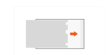
4 Push inner section with installed HDD or SSD into the case.
