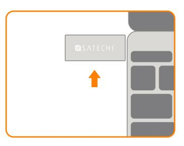
**3.** Connect SD or Micro SD card to the appropriate port of Card Reader.
