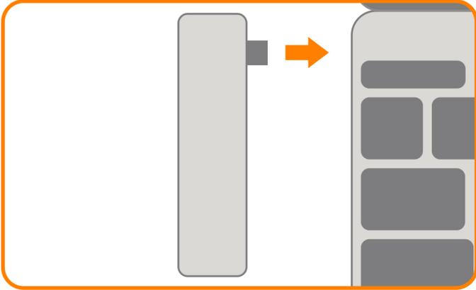
2. When the hub is plugged correctly the **LED** on the hub will turn on.
