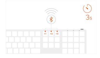
4 To toggle between connected Bluetooth devices, press Bluetooth 1, 2, or 3 button. To remove saved Bluetooth device, press Fn + Shift (left) + Delete.
