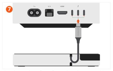
Place the stand on a flat surface and use the USB-C cable to connect to your M4 Mac Mini.
