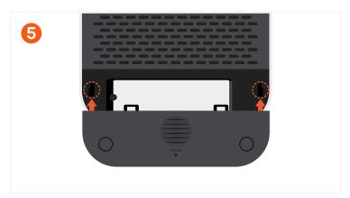
Carefully reattach the enclosure cover: insert the side clips first, then slide the door into place.
