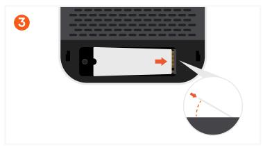
Insert the SSD at a slight angle (35-45°) and ensure it is fully seated in the PCle slot.
