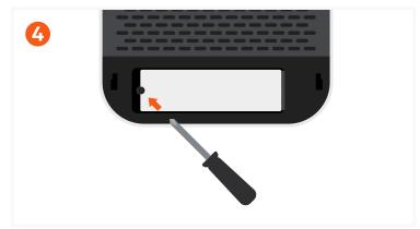
Secure the SSD using the included screwdriver and screw. Tip: To prevent stripping the screw, do not overtighten.
