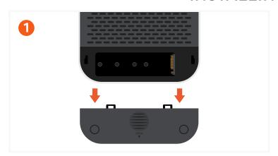
Remove the SSD enclosure cover on the bottom of the stand.
