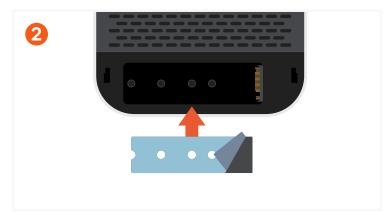
Before installing NVMe SSD, first apply the included thermal tape.
