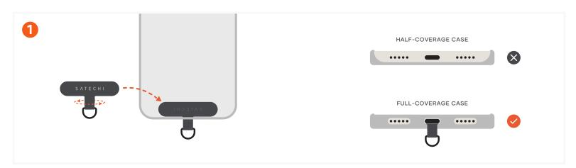
Place the included connector card with the Satechi logo facing the phone case (not included) and insert the loop through the charging port opening.
