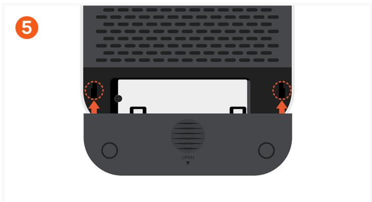
5 Carefully reattach the enclosure cover: insert the side clips first, then slide the door into place.
