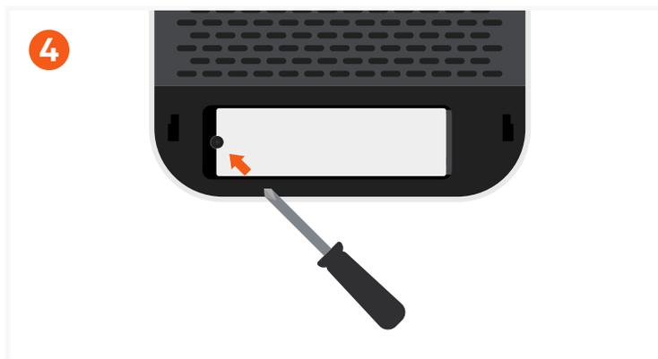
4 Secure the SSD using the included screwdriver and screw. Tip: To prevent stripping the screw, do not overtighten.
