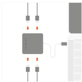
2 Connect up to four USB-C devices for fast data
