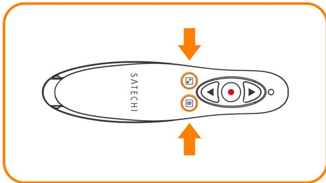
2. To put the Presenter in **Pairing Mode**, press and hold the "Next slide" and "Prev. slide" buttons for **~3 seconds**, then release.
