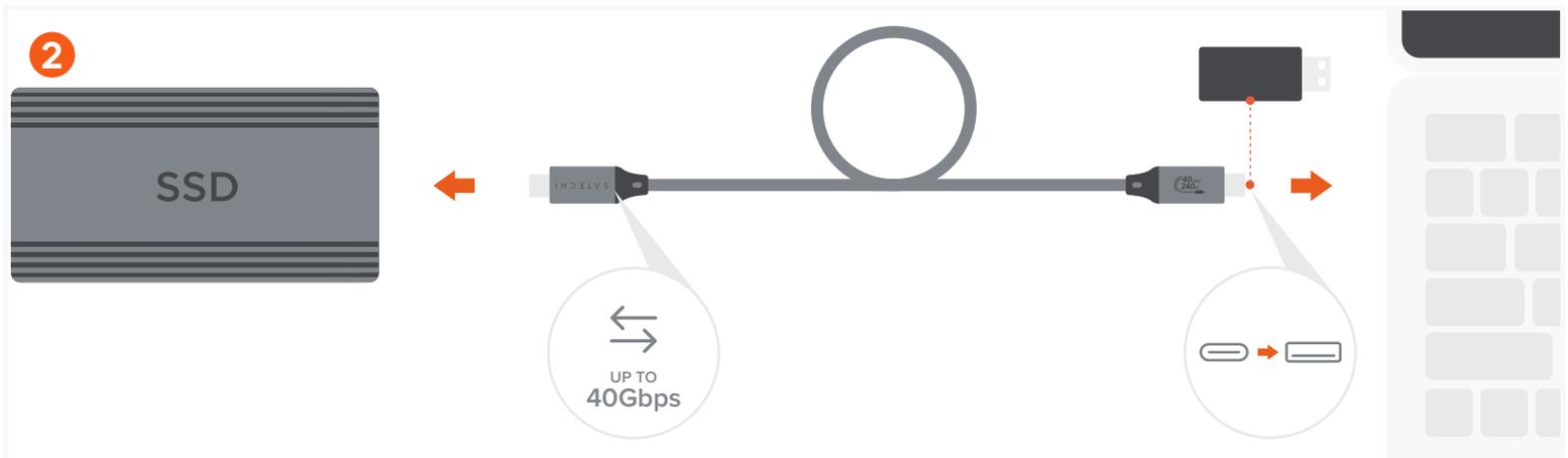
Connect USB4 cable to your USB-C or Thunderbolt 3/4 host devices for fast data transfer speeds up to 40Gbps.
