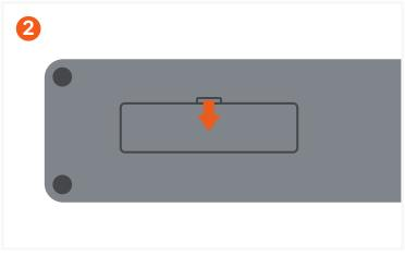
To install the SSD, press and lift the latch on the SSD cover.
