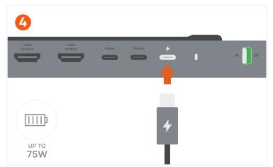
Use the USB-C PD port to charge your device up to 75W. ~15W is used for the docks operation
