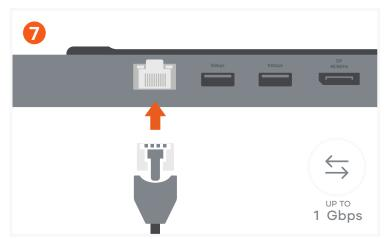
Connect an RJ45 Ethernet cable to the dock's Gigabit Ethernet port. Up to 1 Gbps
