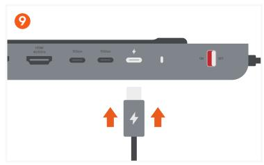
Connect Dual Dock Stand to the power source. Prior to connecting power please make sure all external drives are disconnected from the Dock.
