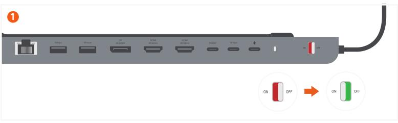
Slide the power switch to the left from red to green in order to turn on the Dock. White LED will turn on signifying the dock is on
