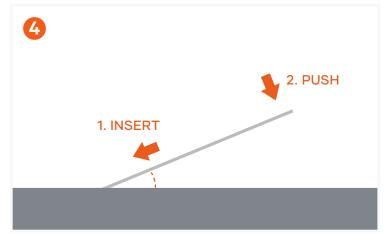
Insert the SSD (not included) at an angle and faceup with the pins aligned and push down to align the SSD with the screw hole.
