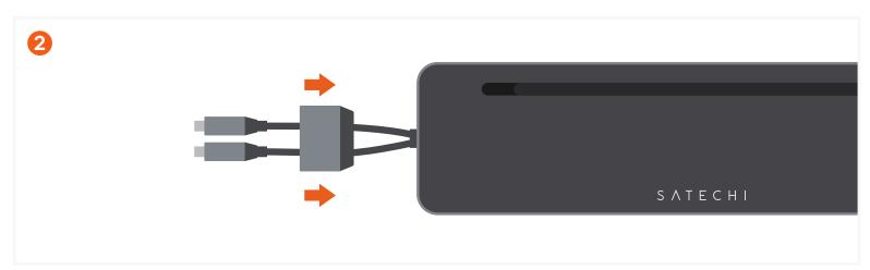
If using with a host device other than a MacBook, slide the aluminum cable cover down to release the cables. Both cables must be connected in order for full functionality
