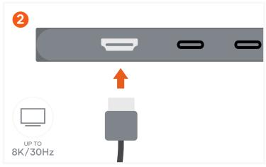
Use the HDMI port to output video to an external monitor or display – up to 8K at 30Hz or 4K at 60Hz/120Hz/144Hz. Computer, cable, and monitor must support 8K. 8K video output not supported on Mac devices.
