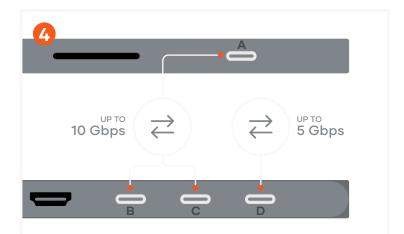
USB-C data ports allow for transfer data at up to 10 Gbps (A, B, C) and 5 Gbps (D) speeds.
