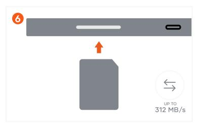
SD card reader supports up to UHS-II read/write speeds.
