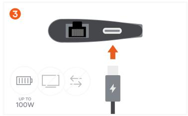
Use the USB-C PD port to charge your device up to 100W. ~15W is used for adapter operation. Video and data transfer not supported.
