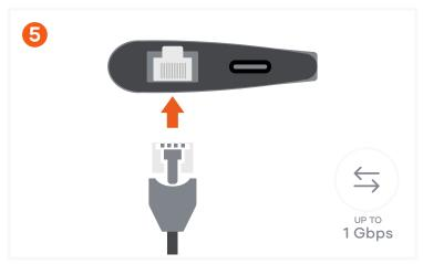
Connect an Ethernet cable to the adapter's Gigabit Ethernet port.
