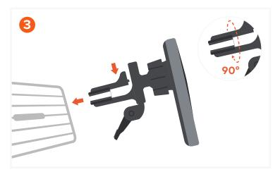
Push the lever to open the clamp and attach onto car's air vents. Rotate clamp 90° to fit onto vertical air vents. Fits most standard car vents.
