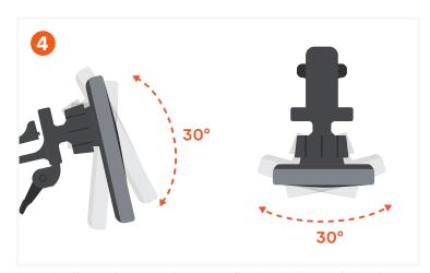
Once the Charger is mounted you can adjust its viewing angle by  $30\,$  degrees.
