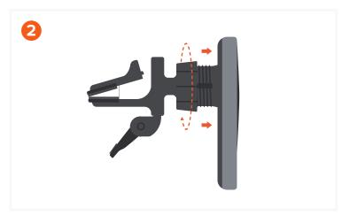
Twist the knob to tighten and secure the two pieces together.
