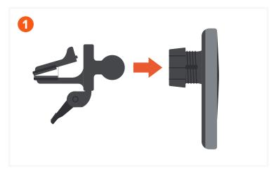
Snap in the mount piece to the backside of the Charger.
