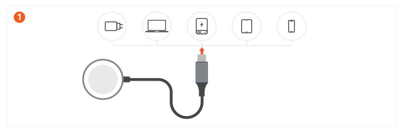
To start charging, please connect the Cable to a USB-C charger or port that provides a 5W output or more.
