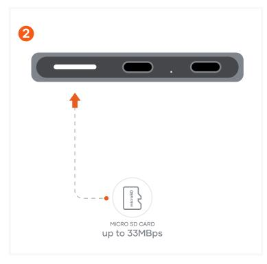
Insert a UHS-I microSD card into the card reader slot. Supports UHS-I SDXC microSD cards.
