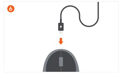
Recharge the mouse using the provided USB-C cable. Up to 45 days of use between charges
