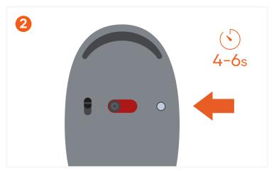
Put the mouse into pairing mode. Press and hold the Bluetooth button for 4-6 seconds. The button will flash blue
