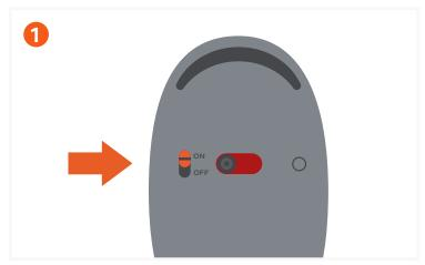
Turn on the M1 Bluetooth Mouse using its backside power switch.
