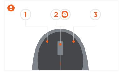
The mouse is equipped with 3 buttons and a scroll wheel.
