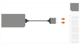
Use HDMI cables to connect up to two HDMI-enabled monitors. One port supports 4K 60Hz and the second 4K 30Hz Requires a direct HDMI to HDMI connection
