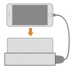
Use 2 Type-C USB ports (5V / 3A) to charge high-powered devices like notebooks.
