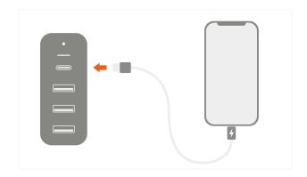
6 Connect your USB-A devices to 2 additional USB 3.0 ports (5V / 2.4 A).
