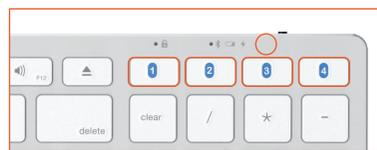
2. Turn on the keyboard power and press the 1 ~ 4 button for about 3 seconds. (Please make sure the blue LED is flashing)
