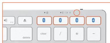
2. Turn on the keyboard power and press the 1 ~ 4 button for about 3 seconds. (Please make sure the blue LED is flashing)
