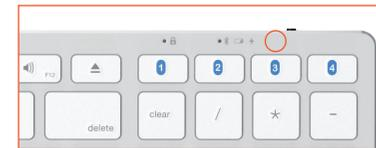
*Note: Please charge the battery before using until the red LED turn off.*
