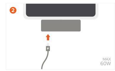
Connect a USB-C Charging cable to the USB-C PD port on the hub to charge your host device (60W Max). Recommended to connect a 30W Power Supply or higher to maintain charging speeds.
