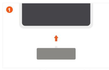
Plug the hub into the USB-C port on your iPad or USB-C host device (requires USB3.1 Gen 2 or higher). Use the included USB-C extension cable for a more stable connection or if using your tablet with a case.
