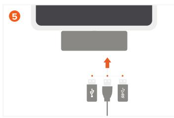
Connect USB peripherals to the USB 3.0 data port. Please update to iPadOS 13 or higher to utilize data transfer to/from external storage devices.
