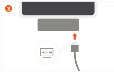
Connect an external display to the hubs HDMI port. Requires a direct HDMI to HDMI connection. Max resolution and refresh rate: 4K at 60Hz.
